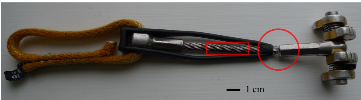
Figure 4: Yellow 1.0, location of failure circled, location of figure 6 marked by rectangle
