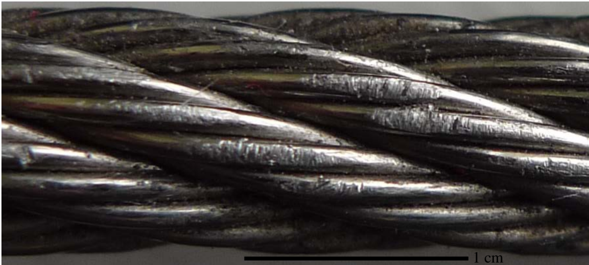
Figure 6: Yellow 1.0 cable abrasion
