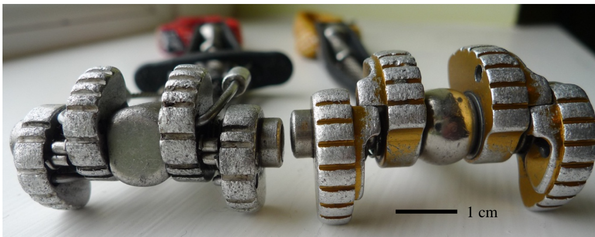
Figure 9: Left Red 0.5, and right Yellow 1.0 cam lobes
